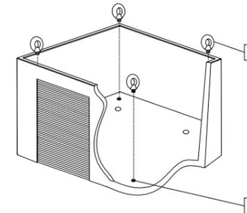
2 elevar mediante eslingas / lifting with slings
