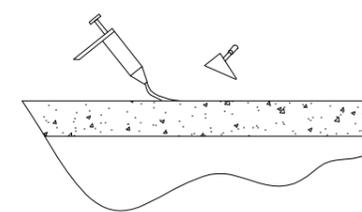
4 instalar sobre la resina epoxy / install over resin epoxy
