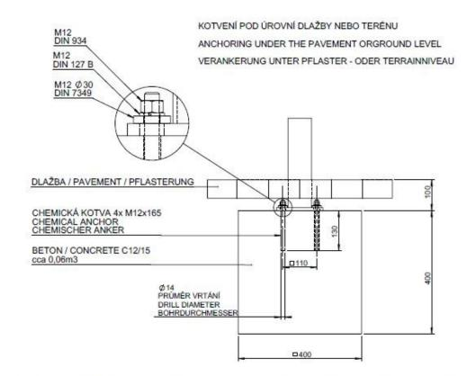
DATE: 13.1.2015 V: 02 minimal load-bearing capacity of the soil 150kPa
