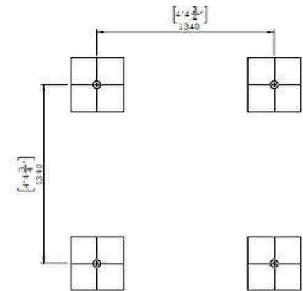
**DETAIL KOTVENÍ, VČETNĚ SPOJOVACÍHO MATERIÁLU, DIMENZE PATEK A HLOUBKY KOTVENÍ, NA VÝKRESE PIXx10-PIXx20\_foundation a PIXx101-PIXx201\_foundation**
