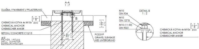
1'1 25 350 DATE: 17.6.2020 V: 00 minimal load-bearing capacity of the soil 150kPa
