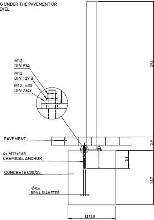
ANCHORING ON THE PAVEMENT
